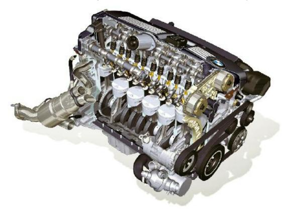
The engine underwent minor modifications in September 2006 and is now designated N52K. With the introduction of the N52K, modifications were made in following areas:
